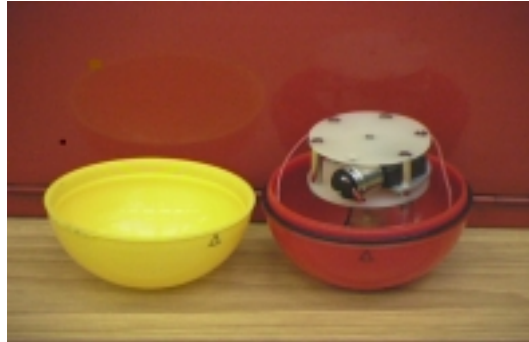
Figure 1 displays the Toni-wha* with the motor in place above the syringe barrel, from this diagram it can be seen that the majority on the space within the robot is to be taken up by the syringe driver and its gear train.
